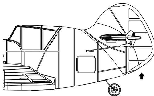
*To be able to fly the aircraft, the ailerons and elevator must be centred. If this is not the case, the respective servo horn must be moved to the centre position. To do this, loosen the screw on the servo head and adjust the servo horn manually. Then tighten the screw again.*
