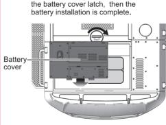
2. Connect the rechargeable battery pack to the power port of the demolition machine closely
