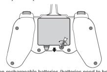
2. Put Three 1.5V AA non-rechargeable batteries (batteries need to be purchased separately) into the battery box to the right polarity at the bottom of remote control.
