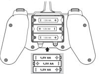
3. Install the battery cover and tighten the screw.
