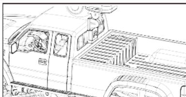
connect the battery pack to the interface of truck body, and close Battery cover.
