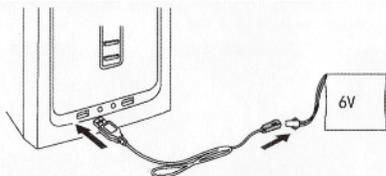
Connect the battery to the charging cable, then plug the USB charging cable into the USB port of the computer or the USB charger. Then turn on the power. When the red light is on, it means that charging is in progress, and when the red light is off it means the battery has been fully charged
