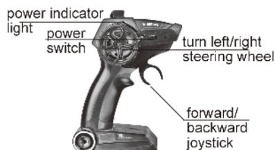
1. When control joystick pull backward, the car will go forward, when control joystick push forward, the car will go backward. When the joystick is pulled back to a half, the car will move forward slowly. When the joystick is fully pulled back, the car will move forward at full speed.
